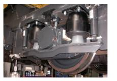
Special rubber ring springs are used for low height wagons travelling on railways with small curvature radius.
