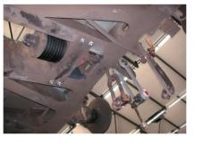
The shock absorbers of the wagon coupling are exposed to very high static and dynamic deformation. The practical tests are endorsed with external laboratories.
