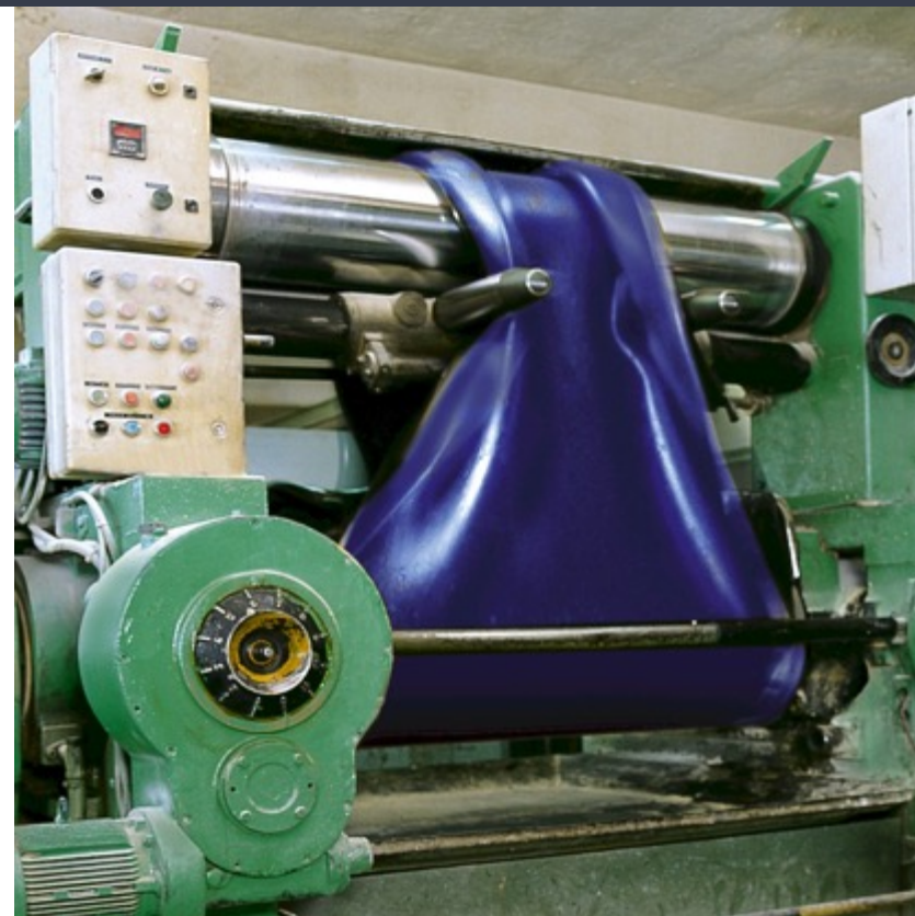
Mixing - open rolling mill
