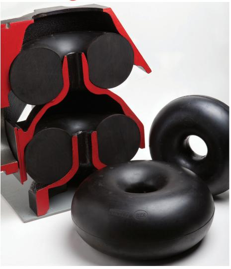
The rubber roller spring can be used in bogies both as primary or as secondary suspension. By using the rubber roller spring suspension for freight wagons, the driving behaviour - even in unfavourable conditions with track defects- is improved and the noise is reduced. By the 3-dimensional design of the suspension the force level for keeping the track is reduced and thus a lower wear level is achieved.
